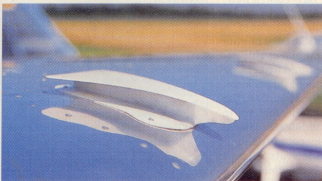
The roomy cockpit, with low side windows and a curved windshield, gives occupants a sense of space (above). Two vortex generators on each wing make the Symphony particularly responsive when approaching a stall (left).
